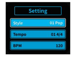
In this interface, press the right encoder to switch between the Style, Tempo, and BPM options. The Style option includes 11 music styles, Tempo switches between 11 rhythm patterns within the selected style, and BPM sets the playback speed of the rhythm pattern, synchronized with the Tap Tempo setting.
