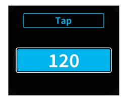
Method 2: In this mode, you can also adjust the BPM by turning the left encoder. If there is no input in this mode for 5 seconds, it will automatically exit and return to the main display, with the left footswitch resuming its Fill function.
