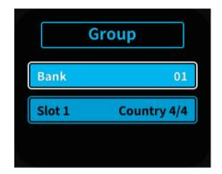
In this interface, press the left encoder to switch between selecting the Bank and Slot options. The FF02 has 11 Bank groups, each with 6 Slot positions. Each Slot can save a rhythm pattern. Use the left encoder to select the desired Bank and switch between Slots within the current Bank.
