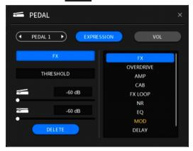
You can set up the function of expression pedal in the current preset patch. Pedal 1 for internal pedal, Pedal 2 for external pedal.
